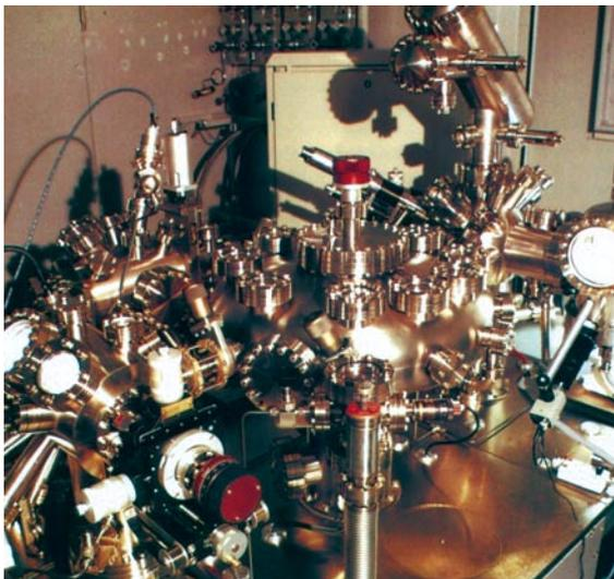
**left:** An Ultrahigh Vacuum chamber housing a scanning tunneling microscope and several other devices for sample preparation and analysis. **middle:** Massive foundations, separated from the building, are necessary to decouple vibrations
