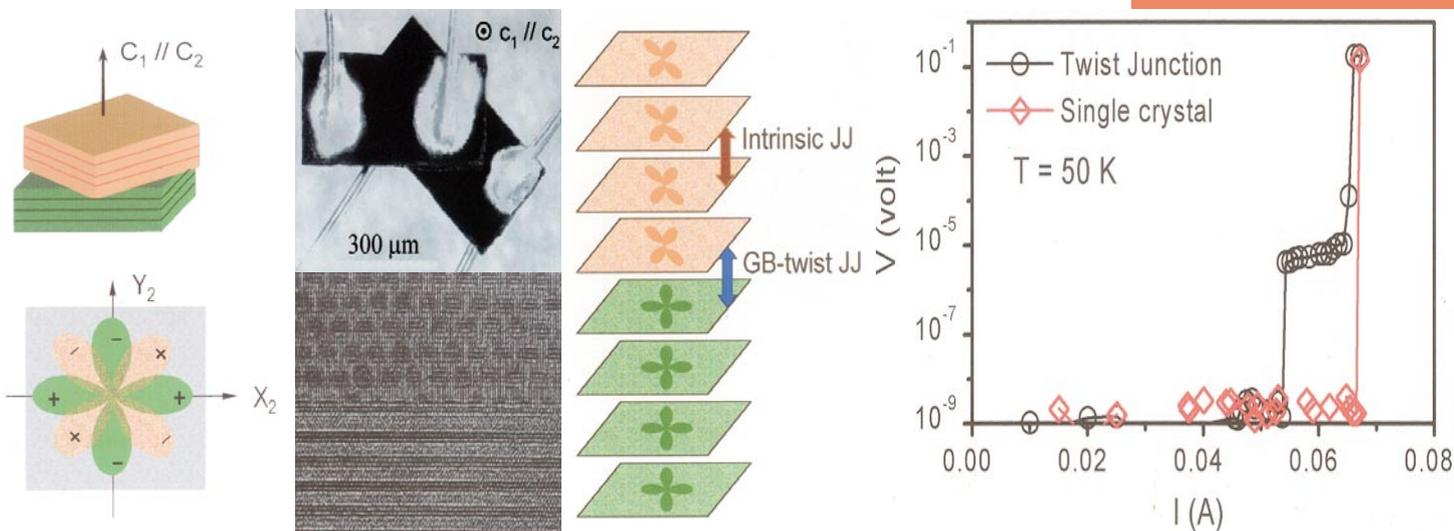
**left:** Schematic representation of a c-axis twist junction of a layered compound and a visualization of the symmetry of a d-wave order parameter above and below the twist grain boundary. **middle:** Top view photomicrograph of a  $45^\circ$  c-axis twist junction, showing three of the six contacts. TEM image of a  $37^\circ$  c-axis twist grain boundary between single crystals of tetragonal  $\text{Bi}_2\text{Sr}_2\text{CaCu}_2\text{O}_{8+\delta}$ . The
