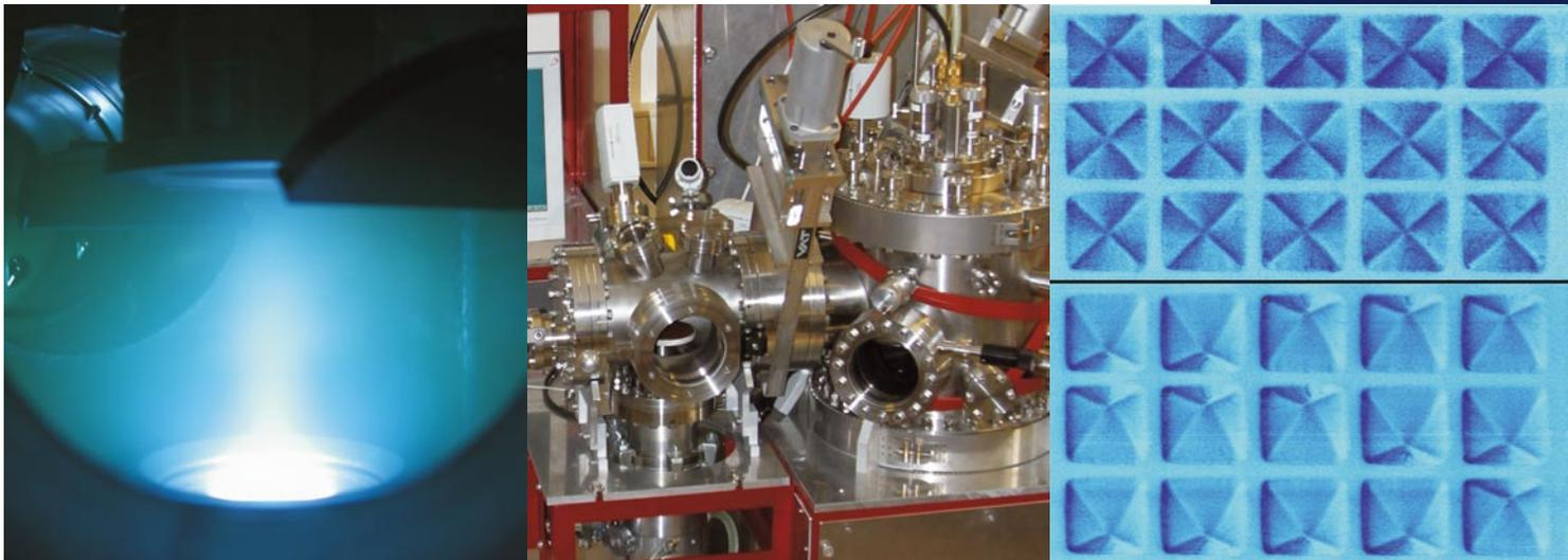
**left:** View into the magnetron-sputtering chamber. An argon plasma is glowing above a permalloy target. **middle:** Magnetron-sputtering plant for ferromagnets, aluminum and copper. **right:**
