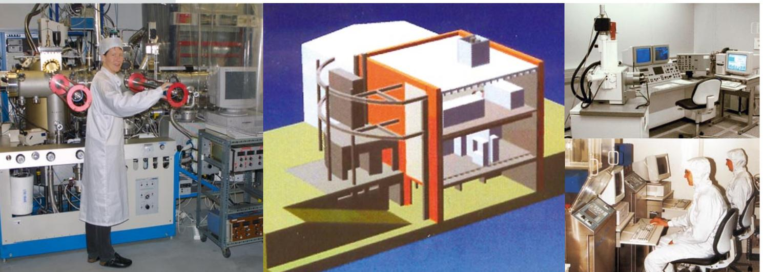
**left:** The molecular beam epitaxy system. **middle:** Sketch of the cleanroom with its three floors for air-conditioning (upper), lab area (middle) and
