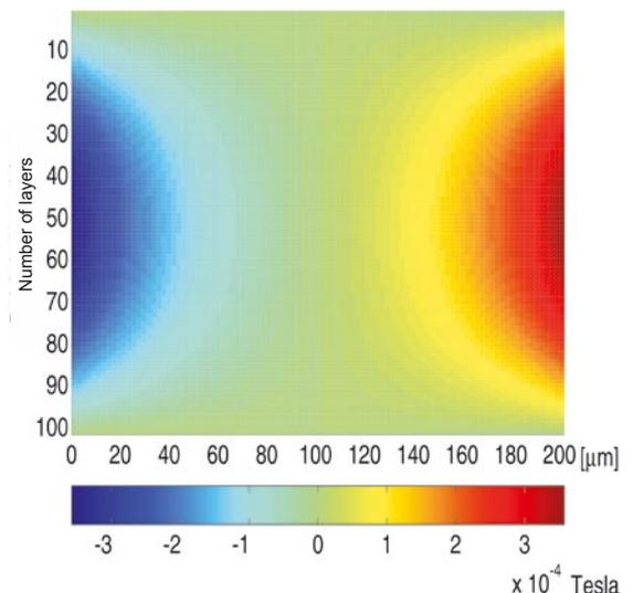
for accelerating particles in high energy physics experiments at DESY. **right:** Magnetic field distribution in a stack of 100 coupled superconducting layers which conducts a current of  $1500 \text{ A / cm}^2$ .
