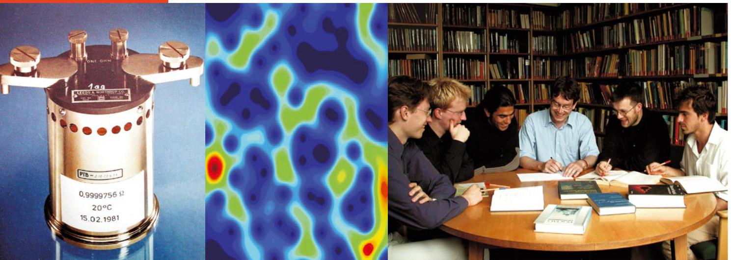
**left:** 1 Ohm, a standard resistance as it was used before the Quantum Hall Effect has been introduced in 1992 as an international standard of the "Ohm". **middle:** A "Swiss Cheese" quantum wave function in a two dimensional random potential landscape,
