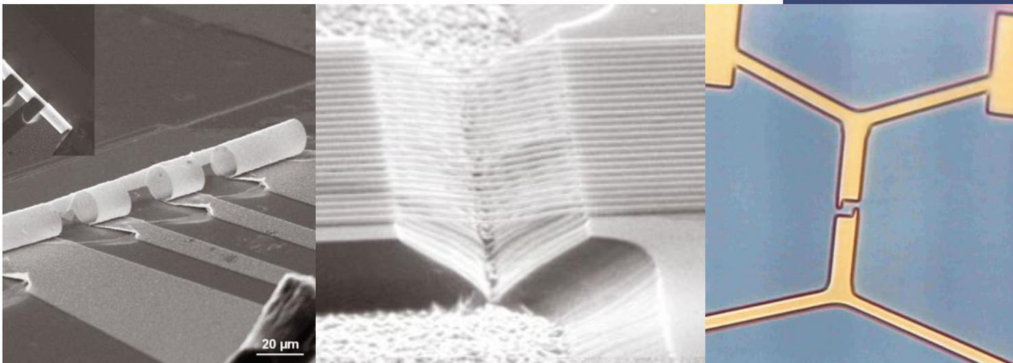
**left:** Semiconductor roll containing a two-dimensional electron system. Light grey stripes are metal pads supplying electrical contacts to the system. **middle:** Free-standing wire bridges that contact gate electrodes of quantum wire
