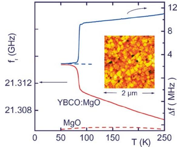
**left and middle:** Switching of the resistance of a 20 nm thin Co-film by a magnetic field directed transverse to the anisotropy field,  $H_A$ , in the film plane. In the longitudinal orientation, the switching is absent. This feature results from the magnetic domain structure, explored by magnetic force microscopy (MFM) shown on the r.h.s. for  $M=0$  and  $H_i=25$  Oe. **right:** Temperature variation of the resonance-frequency
