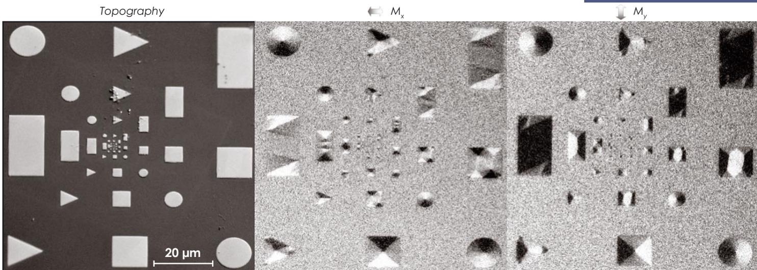
**all 3 fig.:** Topography (left) and domain pattern (middle and right) in Permalloy microstructures obtained by SEMPA. The domain images show the magnetization distribution in two perpendicular
