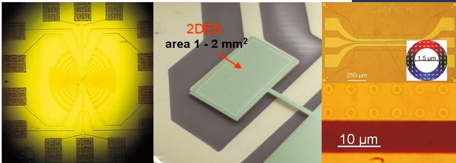
**left:** Antenna structure for focussing far infrared light onto a single quantum wire for photo current spectroscopy. **middle:** Micromechanical cantilever with integrated 2D electron systems supported by a
