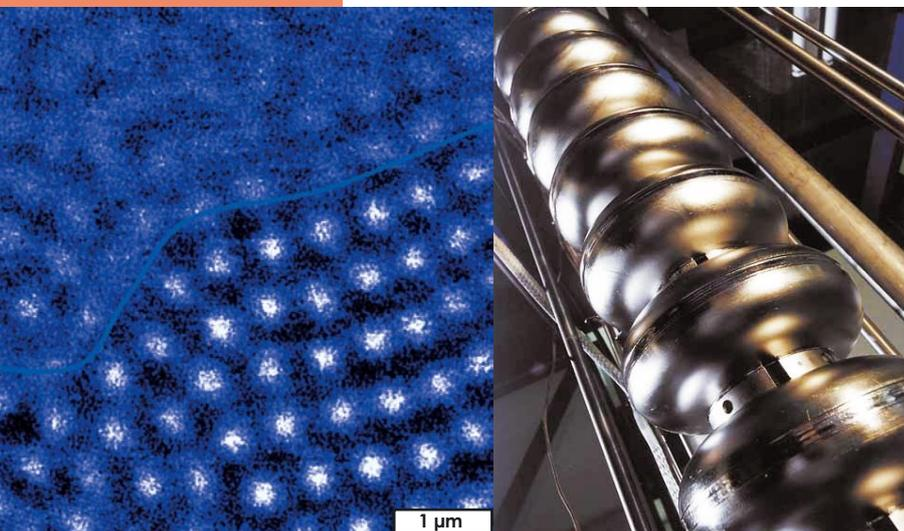
**left:** Abrikosov vortex lattice of  $\text{Bi}_2\text{Sr}_2\text{CaCu}_2\text{O}_8$  with a phase boundary between a solid and a liquid vortex state observed by low-temperature magnetic force microscopy. **middle:** Superconducting cavity
