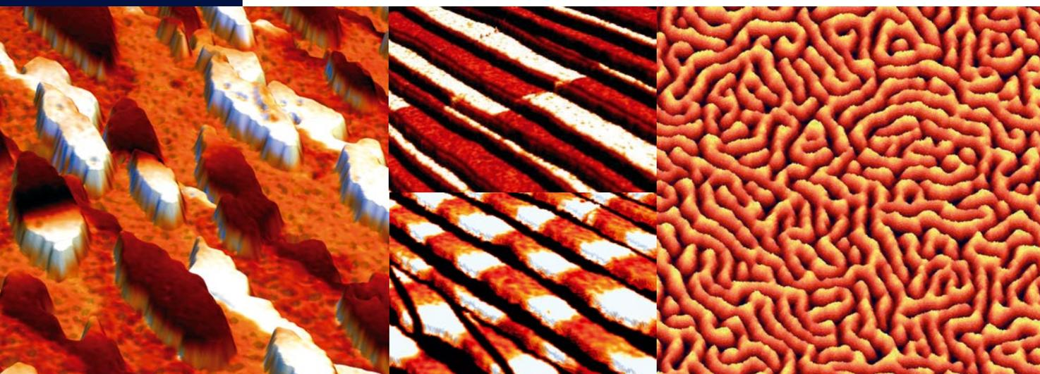
Nano-scale magnetic Fe-islands (**left**) and Fe-wires (**middle**) grown on a stepped W(110) surface. The magnetization directions are color coded and have been determined by spin-polarized STM.
