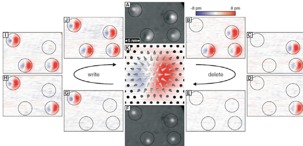
Figure 3.12: SP-STM measurements of a group of isolated skyrmions in the system of the PdFe bilayer on Ir(111) at  $T = 4$  K,  $B = 3.25$  T. Constant-current images (gray-scale) with (A) and without (F) skyrmions pinned at the four defects. The difference images (color-scale, with respect to (F)) show how the skyrmions can be deleted and written independently. The central image depicts the magnetization direction within a skyrmion.
