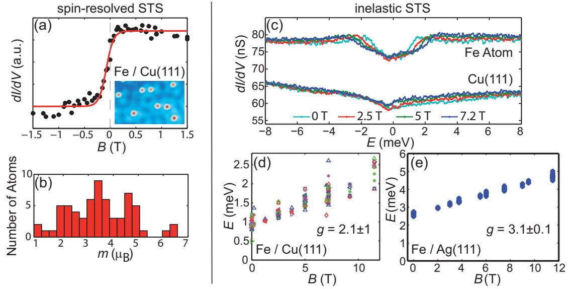
Figure 3.1: Fe atoms on Cu(111) and Ag(111): (a) Magnetization curve of an Fe atom on Cu(111) (black) and fit to a Langevin model (red). (b) Histogram of the fitted magnetic moments [1]. (c) ISTS spectra of an Fe atom and of the Cu(111) substrate at different magnetic fields as indicated. (d,e) Spin excitation energy as a function of the  $B$ -field for Fe atoms on Cu(111) [1] and on Ag(111) [2]. The  $g$ -factors determined from the slope are indicated.
