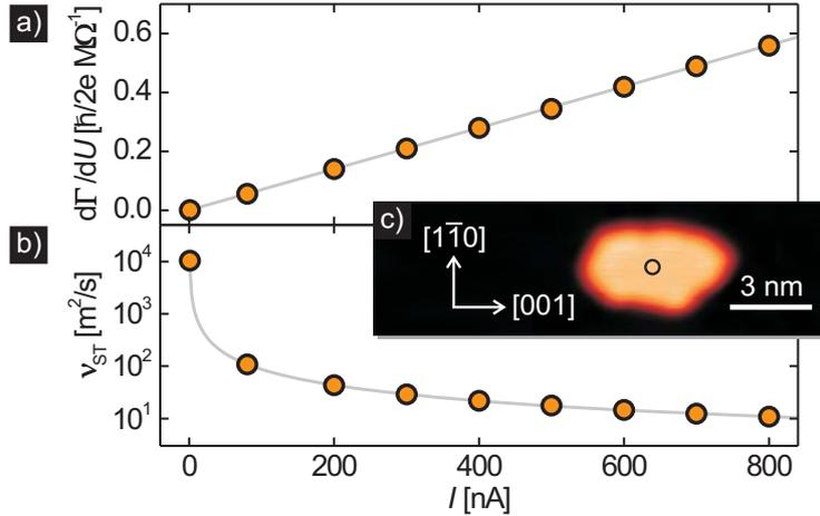
Figure 3.15: Experimentally determined tunnel current dependence of the (a) torkance  $d\Gamma/dU$  and (b) spin-transfer torque viscosity  $\nu_{\text{ST}}$ . Gray lines are guides to the eye. (c) Topography map of the nanoisland. The point of current injection is marked by a circle.
