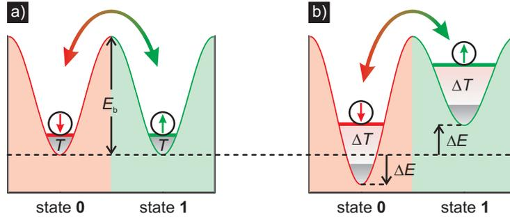
Figure 3.13: (a) Energy landscape schematics of a magnet with uniaxial anisotropy. Due to thermal agitation at temperature  $T$ , the magnetization may overcome the effective activation barrier  $E_b$  between the two states **0** and **1**. (b) Influence of a high spin-polarized current: Joule heating effectively increases  $T$  by  $\Delta T$ , and spin-torque modifies  $E_b$  by  $\pm \Delta E$ , thereby lifting the state degeneracy and favoring switching from state **1** to state **0**.
