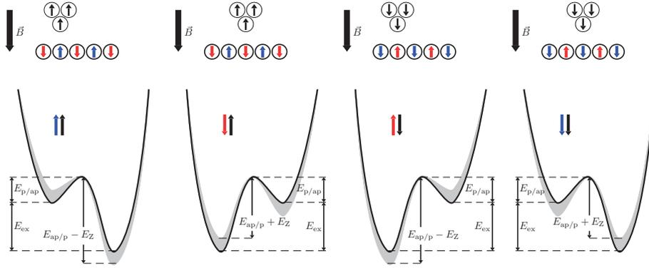
Figure 3.34: Combined effect of an external magnetic field and the magnetic exchange energy between tip and sample on the energy landscape. Note that the magnetic exchange energy is much larger than the Zeeman energy. Since the ap-configuration is energetically favored, only p to ap switching events are observed. Due to the Zeeman energy, the state with the tip apex magnetization parallel to the external magnetic field is preferred.
