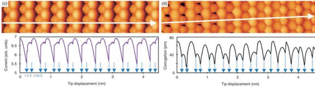
Figure 3.9: Occurrence of spin friction during manipulation of a magnetic adatom. MC simulation (left) and experimental SP-STM image of the Mn-ML on W(110) with a Co atom trapped in the tunnel junction; the blue arrows in the line profiles (bottom) highlight the deviation of the jump positions of the adatom from the equidistant atomic periodicity.
