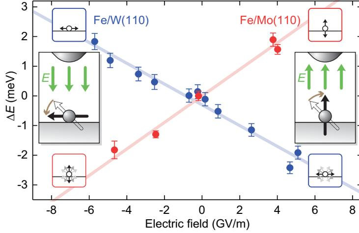
Figure 3.28: Electric field dependent energy barrier variation for an in-plane (Fe/W(110)) and an out-of plane (Fe/Mo(110)) system. Negative electric fields favor in-plane, positive electric fields out-of plane orientation of the magnetization.
