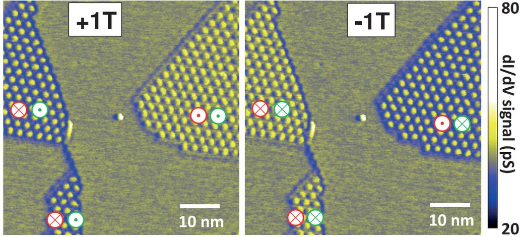
Figure 3.52: Out-of-plane magnetic maps of the intercalation regions. Spin-resolved  $dI/dV$  maps ( $-0.9V$ ,  $1nA$ ) acquired with an applied out-of-plane magnetic field a)  $+1T$ , b)  $-1T$ . Green symbols: magnetic orientation of the SP-STM tip, red symbols: magnetic orientation of the intercalation regions.
