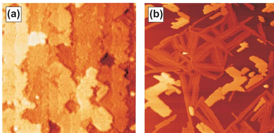
Figure 3.56: (a)  $(200 \times 200)$  nm<sup>2</sup> AFM image after deposition of several monolayers of Co-Salen molecules on NiO(001) at room temperature showing layer-by-layer step-flow growth. (b)  $(2 \times 2)$  μm<sup>2</sup> AFM image after deposition of several monolayers of Co-Salen molecules on NaCl(001) at room temperature exhibiting a biomodal island growth composed of compact nanocrystallites and long nanowires.
