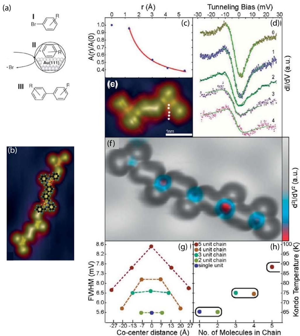
Figure 3.45: (a) Schematic depiction of the Ullmann reaction used to polymerize the individual Co-Salophene-Br into a multi-spin-center macro molecule. Topograph of the molecular Kondo chain with the molecular structure superimposed. Evaluating the Fano resonance arising from the Kondo effect on different macro-molecules (c)-(f). Dependence of the Kondo temperature on the molecular chain length showing a clear even/odd dependence (g) and (h).
