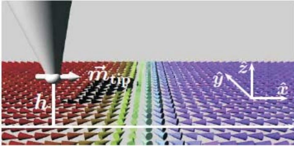
Figure 3.41: Scheme of the initial spin configuration of the sample. A DW elongated in  $y$ -direction separates two domains. The spins in the domains point along the easy-axis with blue ( $-x$ ) and red colored cones ( $+x$ ). A tip with a magnetization  $\vec{m}_{\text{tip}}$  and distance  $h$  from the sample moves towards the DW on the indicated track (white dashed line).
