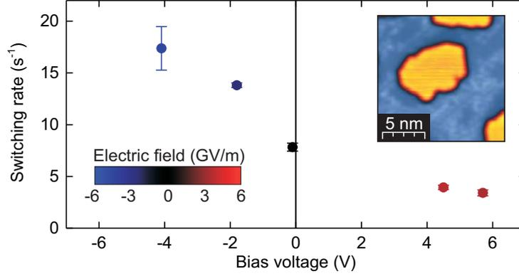
Figure 3.27: Switching rate as a function of applied bias voltage for the Fe/Mo(110) nanomagnet. Data points are color coded with the electric field strength.  $I = 100$  pA,  $T = 26.5$  K. The inset shows the topography of the island.
