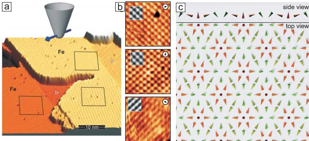
Figure 3.6: The system of one monolayer Fe on Ir(111). (a),(b) SP-STM measurements of all possible rotational magnetic domains imaged with an in-plane sensitive tip. (c) Sketch of the derived commensurate magnetic structure: the nanoskyrmion lattice is nearly square with a periodicity of about 1 nm.
