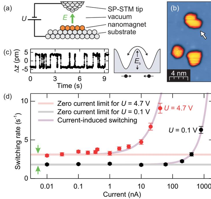
Figure 3.24: (a) Scheme of the experimental setup. (b) Spin-polarized STM topography taken at  $U = -100$  mV,  $I = 2$  nA,  $T = 45$  K. (c) Telegraph signal observed when the tip is positioned above the island marked in (b) and scheme for thermal magnetization reversal. (d) Switching rate of the island as a function of tunnel current for two different bias voltages (lines are guides to the eye).
