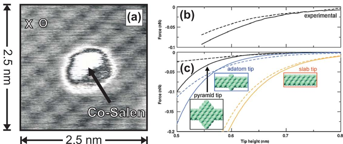
Figure 3.54: (a) Atomically resolved NaCl(001) imaged together with a single Co-Salen marker molecule using a metallic Cr-coated tip. Protrusions correspond to Cl-sites. X and O indicate the location of the two experimental spectroscopy curves shown as solid and dotted line, respectively, in (b). Simulated force curves for each of the three tip models (see insets: blunt, single adatom and three layer pyramid, respectively) above Cl and Na ions are shown in (c).
