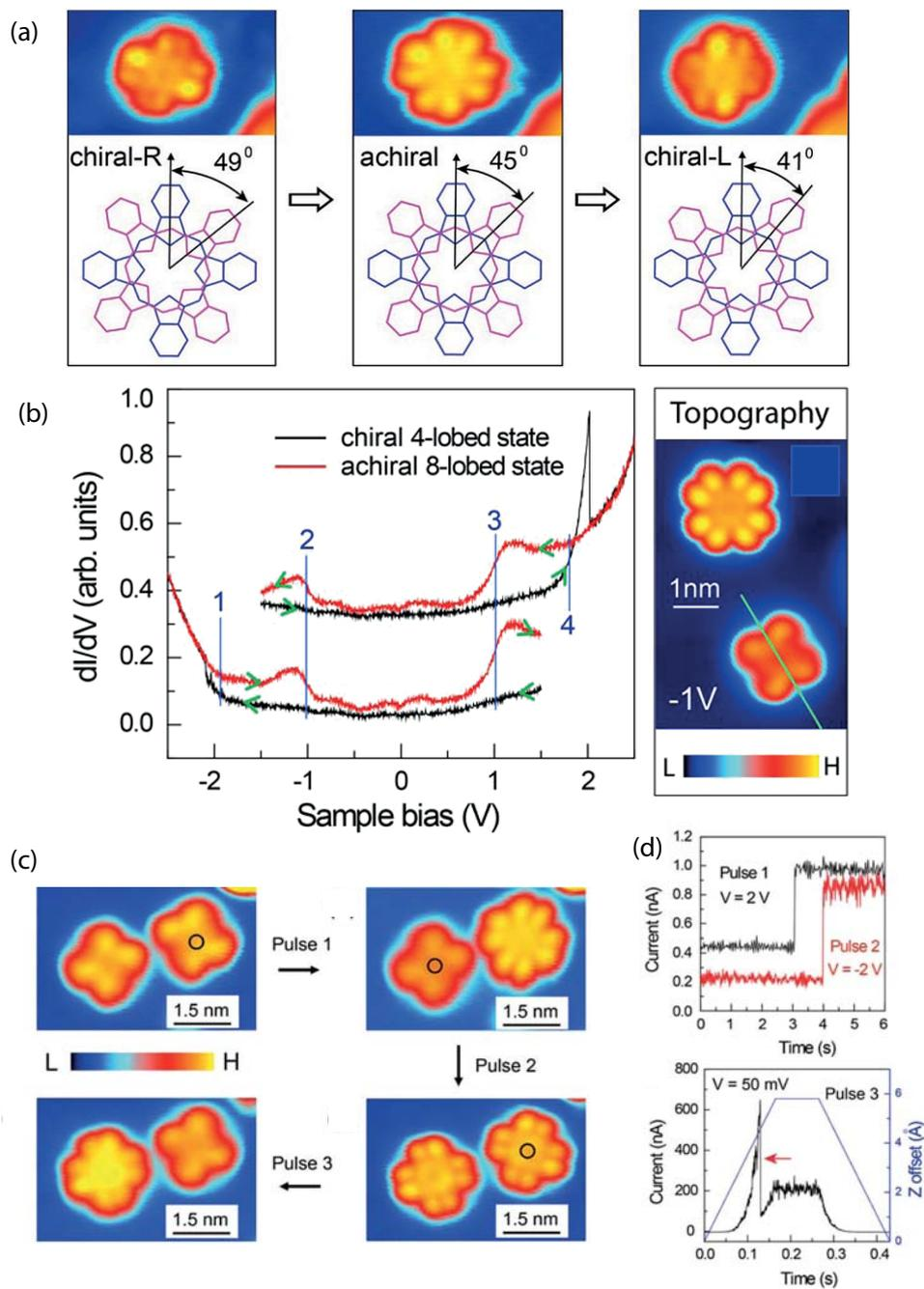
Figure 3.49: Reversible STM induced switching of TbPC2 molecules on Ir(111). TbPC2 can be switched between a chiral and an achiral state(a). The STS signature of the achiral and chiral state, respectively (b). A controlled manipulation sequence (c) demonstrating the interconversion between states *via* the manipulation protocols given in (d).
