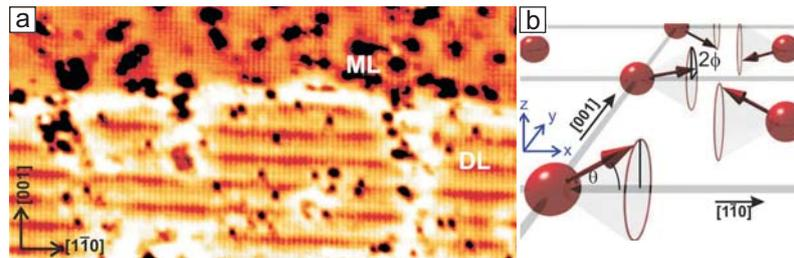
Figure 3.8: Conical spin spiral of the Mn-DL on W(110). (a) SP-STM image of ML and DL connected at a buried W step edge. The DL shows a two-atom magnetic periodicity along  $[1\bar{1}0]$  and a larger modulation along  $[001]$ . (b) Model of the conical magnetic state.
