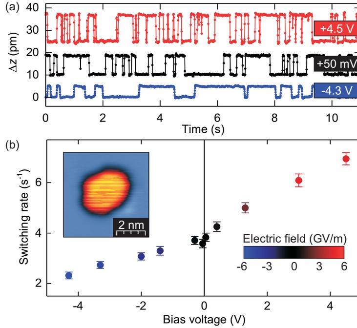
Figure 3.25: (a) Time traces recorded at different bias voltages. Curves were offset for clarity. (b) Switching rate as a function of applied bias voltage. Data points are color coded with the electric field between tip and sample. All measurements were performed at  $I = 100$  pA,  $T = 45$  K. The inset shows the topography of the investigated island.
