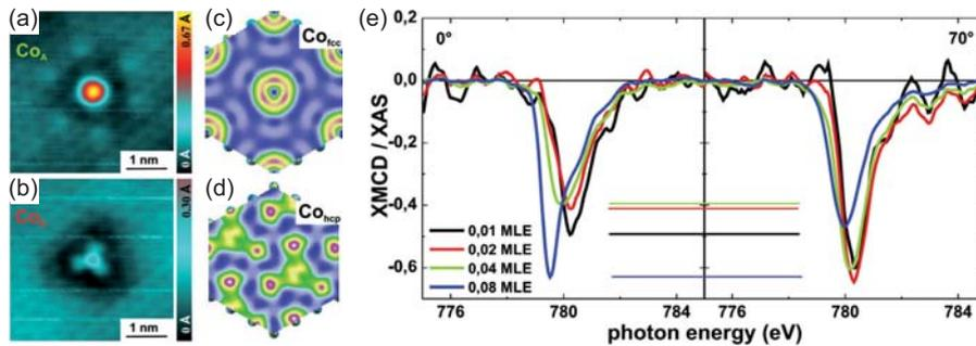
Figure 3.65: (a), (b) STM topograph of two different types of isolated Co adatoms on  $\text{Bi}_2\text{Se}_3$  showing the affected surface in their vicinity. (c), (d) Simulations of Co atoms adsorbed in the fcc and hcp hollow site. (e) Normalized XMCD signals for a series of coverages ranging between 0.01 ML and 0.08 ML for normal (left panel) and grazing (right panel) incidence angle. The colored lines are guidelines to the eyes indicating differences between both angles [6].
