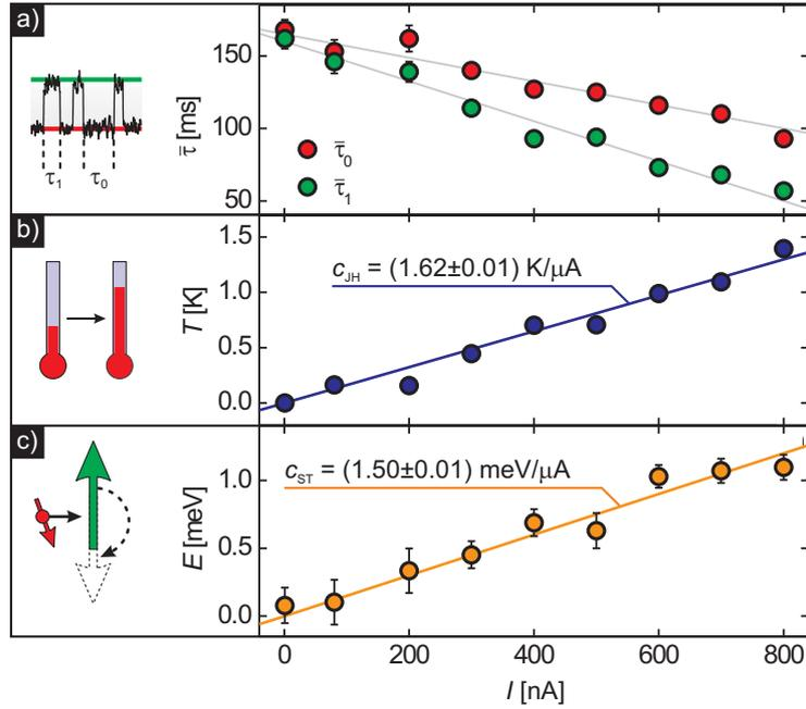
Figure 3.14: Tunnel current dependence of the (a) mean lifetimes  $\bar{\tau}_0$  and  $\bar{\tau}_1$  (gray lines are guides for the eye), (b) effective island temperature increase  $\Delta T$  and (c) energy barrier modification  $\Delta E$ . Error bars indicate SD. Linear fittings yield the coefficients  $c_{\text{JH}}$  and  $c_{\text{ST}}$ .  $U = -200 \text{ mV}$ ,  $T = 50.6 \text{ K}$ .
