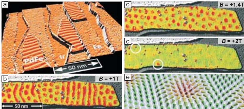
Figure 3.11: SP-STM measurements of the system of the PdFe bilayer on Ir(111) in dependence on an external magnetic field at  $T = 8$  K. (a)  $B = 0$  T: spin spiral state, (b)  $B = 1$  T: coexistence of spin spiral and skyrmions, (c)  $B = 1.4$  T: hexagonal skyrmion lattice, (d)  $B = 2$  T: ferromagnetic phase. (e) Sketch of the magnetic skyrmion lattice phase.
