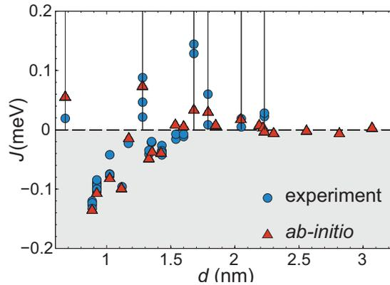
Figure 3.3: Distance dependency of the RKKY interaction in pairs of Fe adatoms on Cu(111). Measured (blue circles) and KKR-calculated (red triangles, renormalized by a factor of  $1/2$ ) exchange energy  $J_{ij}$  in pairs of Fe atoms on Cu(111) as a function of separation. [5]
