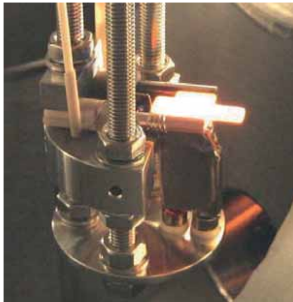
Figure 3.78: An empty sample tray being heated by electron bombardment. Grooves in two tungsten rods receive the sample tray or the tip transporter. The electron-emitting filament is positioned right underneath the tray. With the tungsten rods held at high positive voltage, the electrons get accelerated and release their kinetic energy upon impingement on the tray's back side.
