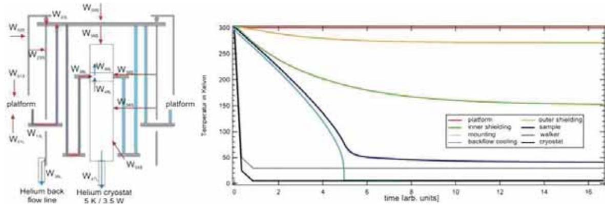
Figure 3.79: Left: schematic representation of the experimental setup and paths of heat dissipation. The numerical modeling covers heat radiation ( $W_{xyS}$ ) and heat transport ( $W_{xyL}$ ) between the different parts of the STM setup. The right graph indicates the time-dependent temperature variations for the different parts of the setup after start of the cooling at the time = 0.
