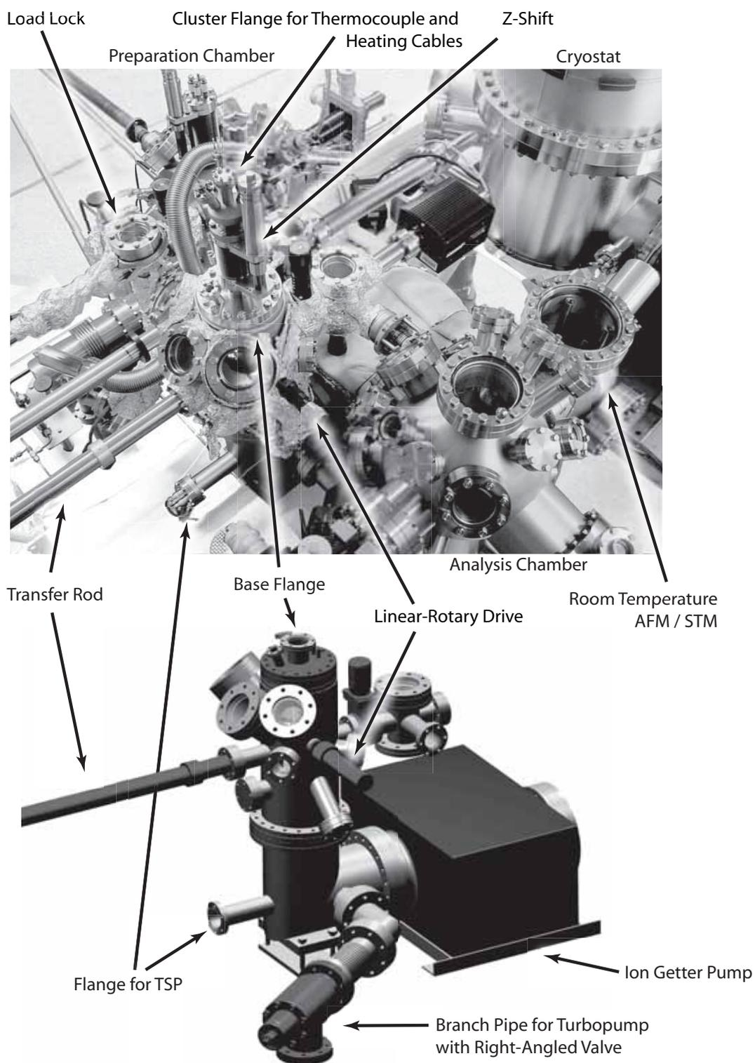
Figure 3.86: Picture of the UHV system with the implemented molecule evaporation chamber. Samples and crucibles can be transferred into the molecule evaporation chamber using the load lock and several transfer rods.
