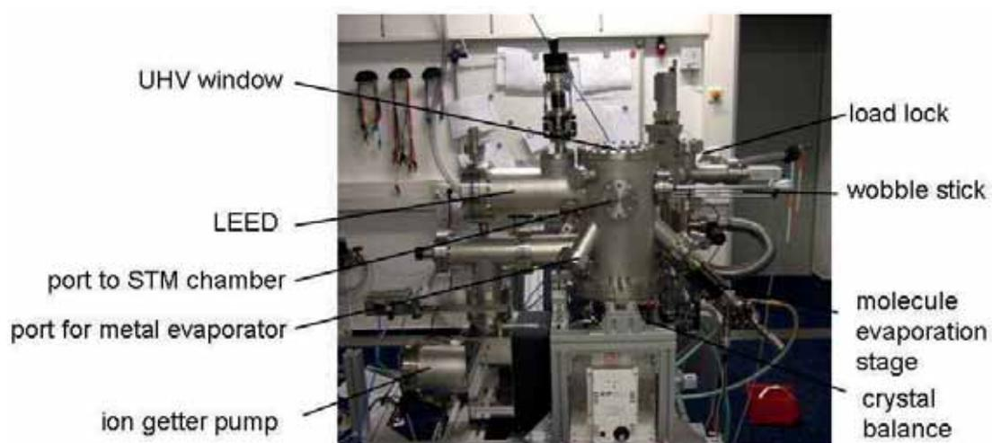
Figure 3.83: Side view of the preparation chamber fixed to a rigid frame which will also host the cryostat system.
