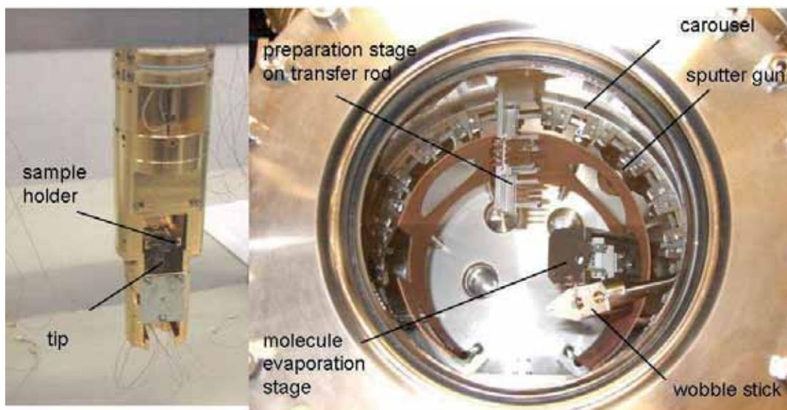
Figure 3.82: (left) Image of the STM head for the new 300 mK system mounted on an ex-situ test stage. A test sample as well as a tip are introduced for first calibration experiments under ambient conditions. (right) Top view into the preparation chamber equipped with most relevant parts. Currently, only the metal evaporators are still missing and testing of the different components is ongoing.
