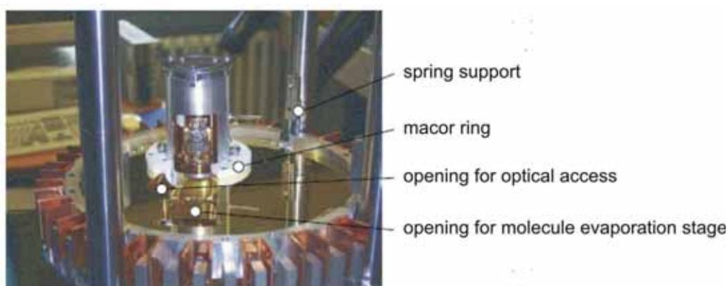
Figure 3.78: Image of the VT-STM head. The STM head is mounted on an eddy current damping stage by Omicron. The gold-plated copper platform is additionally modified to host the self-made STM and enables the integration of a molecule evaporator.
