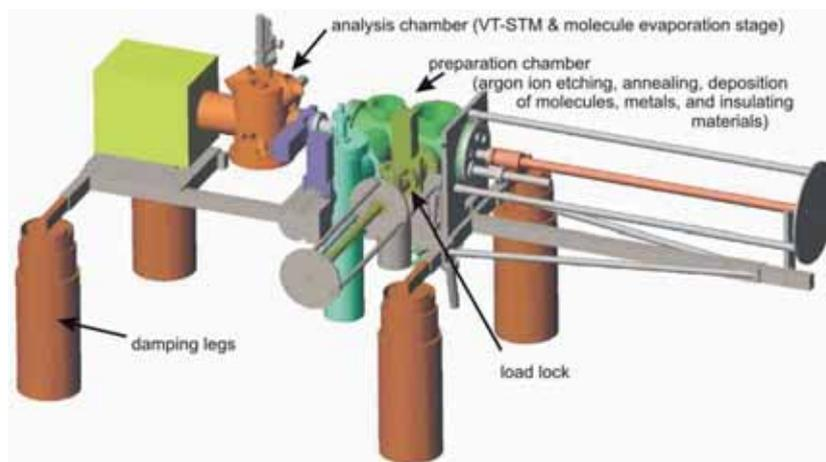
Figure 3.77: 3D-sketch of the ultra-high vacuum system for the preparation and characterization of volatile molecules. The system consists of a load lock to introduce samples, tips, and molecule evaporators, and a preparation chamber to sputter and anneal metallic crystals and to prepare thin layers of molecular, insulating, and magnetic films. The system is completed by the analysis chamber equipped with a VT-STM and a heating stage to deposit molecules with the sample loaded in the cooled STM.
