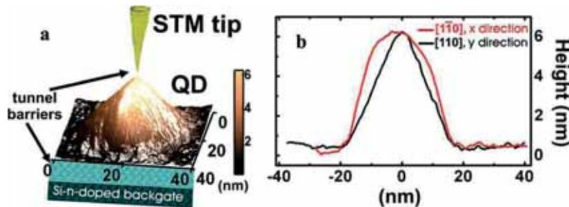
Figure 3.70: **Experimental setup and dot morphology.** (a) Experimental setup and three-dimensional STM image of a representative uncapped QD grown on a n-doped GaAs(001) substrate. (b) Height profiles of the same QD along two perpendicular axes, parallel to the  $[110]$  and  $[1\bar{1}0]$  directions, respectively.
