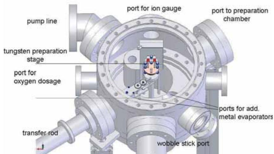
Figure 3.84: An extra side chamber for the high-temperature preparation of tungsten crystals was developed. In this setup other vacuum components are protected against the heat load during the preparation by a water-cooled shield. For temperature measurements optical access for a pyrometer is granted from the top view port.
