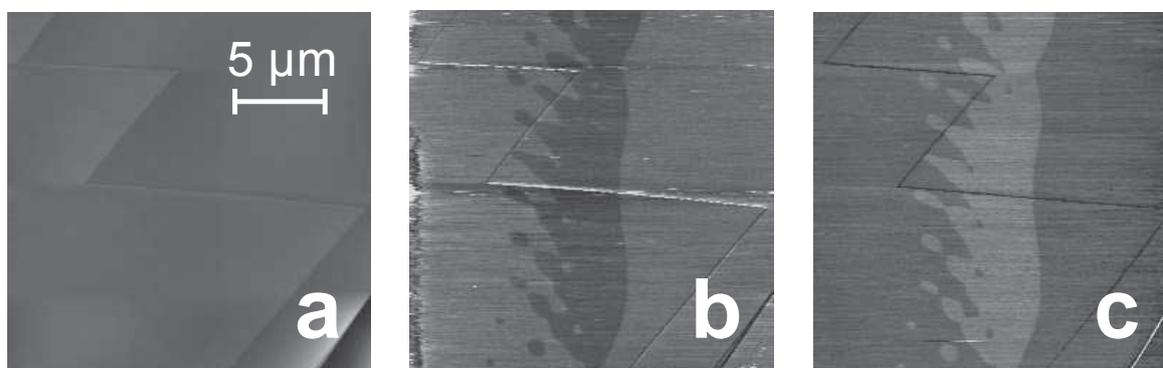
Figure 3.39: **a** Topographic image of the GASH (0001) surface, scan size:  $20 \mu\text{m} \times 20 \mu\text{m}$ ; **b** Forward friction scan image for the same area, **c** Backward friction scan image.
