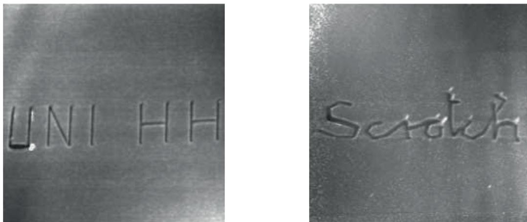
Figure 3.54: Two test patterns written mechanically into a niobium thin film by using an SFM with a diamond tip.
