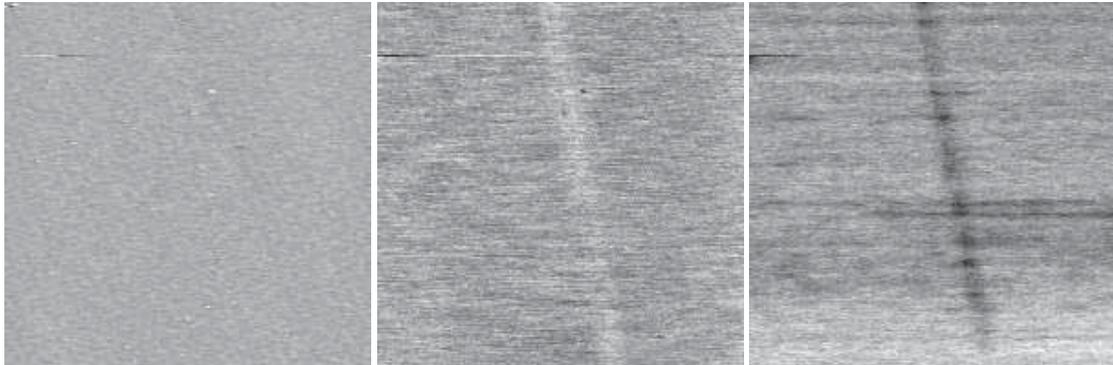
Figure 3.50: Simultaneously recorded topographic, capacitance and  $dC/dU$ -image of the same area ( $35 \times 35 \mu\text{m}^2$ ) of a NOS heterostructure sample. A subsurface defect shows up in the  $C$ - and  $dC/dU$ -images but remains invisible in the surface topographic image.
